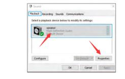
2) Click the loudspeaker is being used-"Properties"--"levels", drag progress bar to adjust volume of output
