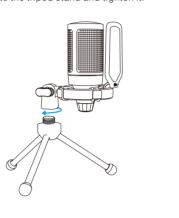
2. Adjust the angle of the mic with the thumbscrew.
